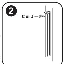
Install second screw (**C**) in top of hinge 2. bracket securing it to the wall.
