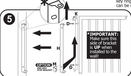
Mount latch assembly (**K**) to gate using 3/4" bolts with serrated washers (**D**). Attach wall mount for latch assembly (**H**) up into part (**K**) that is now secure on gate. Slide gate out to mark holes for (**H**) on attaching wall. (\*OPTIONAL ONE WAY 5. BRACKET INSTALLED HERE) Then attach the wall mount of latch assembly to wall using Phillips head screws (**C**). Optional long screws (J) maybe be used to attach gate to stud through dry wall.
