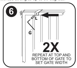
Keep gate closed and latched. Use Allen wrench (G) to insert set screws (L) in the upper and lower brackets of the gate. Tighten the set screws to set the width of the gate.
