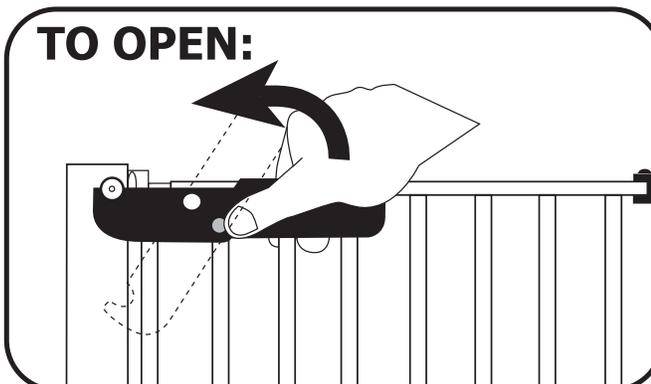
Push red safety button and lift handle 90° upwards. Pull gate to open.
