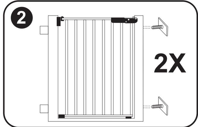
2. Screw stabilizer pads (B) into opposite side of gate. These pads will fit into C-channel of door frame.
