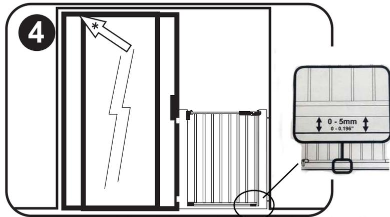
4. Screw door stop (C) to sliding track to secure sliding door (\*). Make sure gate is installed between 0 to 5mm (0 to 0.196in) from floor. The gate shall close to the door frame before use.
