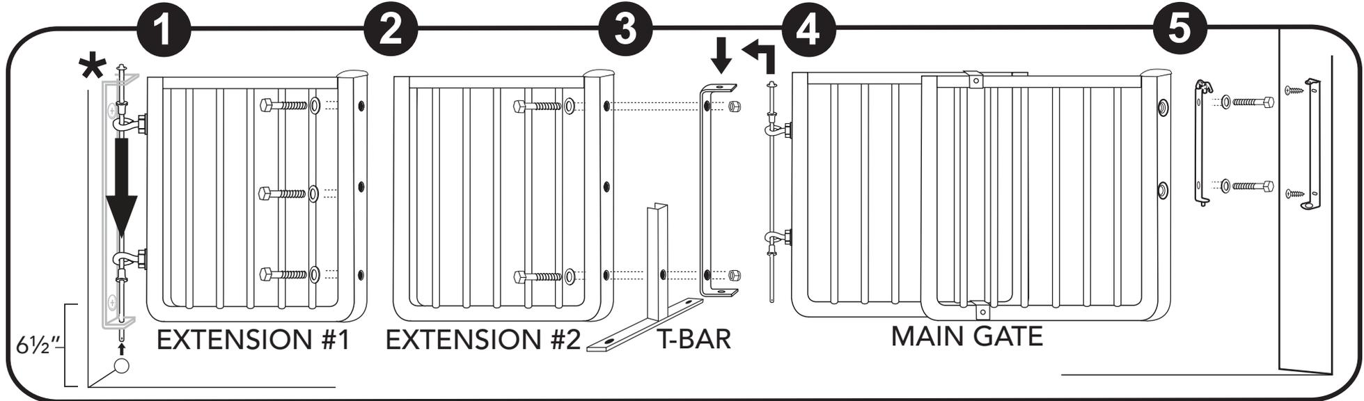
**1 Use Hinge Bracket from Gate Box\*.** Drill a 1/8" pilot hole 6 1/2" from the floor. Secure hinge bracket to wall with screws from the gate box hardware pack. Attach eyebolts from the gate box to the upper and lower threaded inserts on one of the extension with nuts and washers.
