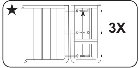
To install the extension, attach extension to gate BEFORE STEP 3 on Model SS-30 or MG-15 assembly instructions.
